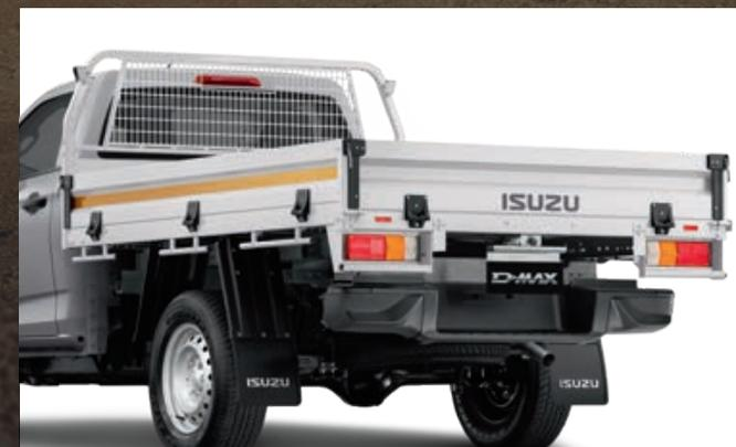
**Mine Specification Steel Tray<sup>#</sup>** - A sturdy steel tray with reflective side striping, a steel mesh window protector and headboard aerial mounts. Available in Mineral White only.
