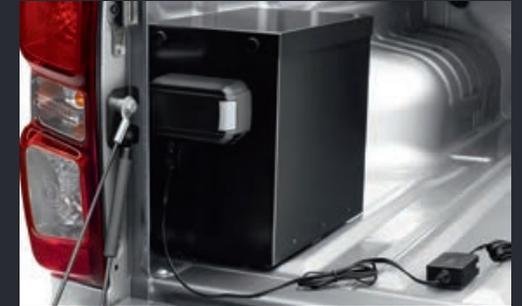
**Dual Battery System & 12V Dual Smart Socket**
